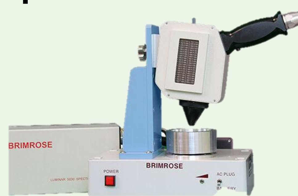
Luminar 5030 NIR analyzer (Brimrose Corporation, Baltimore, USA)
