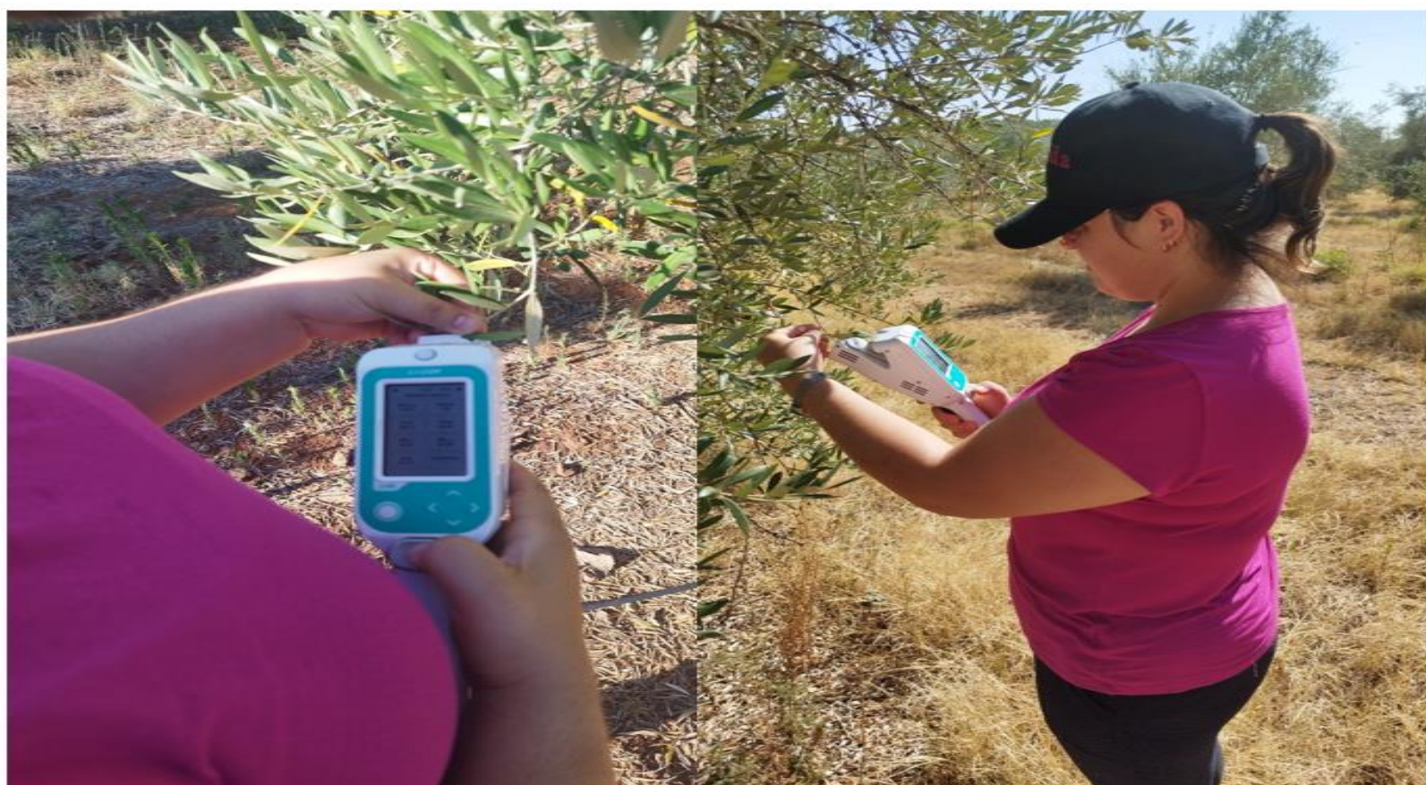
Fig. 1 - Non-destructive measurements with the Porometer / Fluorometer LI-600 in olive tree ( Olea europaea L.) leaves ('Galega Vulgar' and 'Picual' varieties), under irrigated and rainfed conditions.
