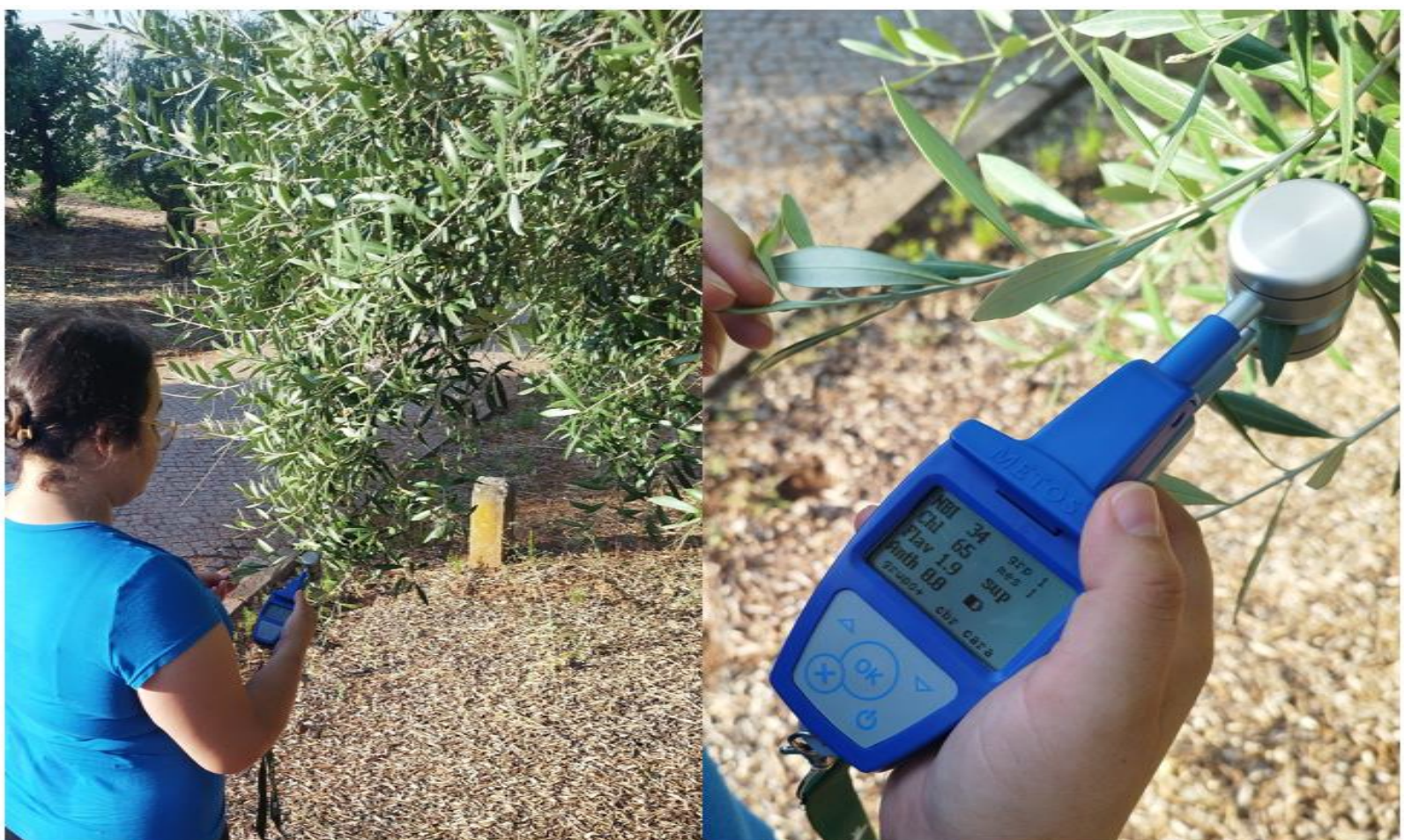
Fig. 2 - Non-destructive measurements with the Dualex leaf clip in olive tree ( Olea europaea L.) leaves ('Galega Vulgar' and 'Picual' varieties), under irrigated and rainfed conditions.
